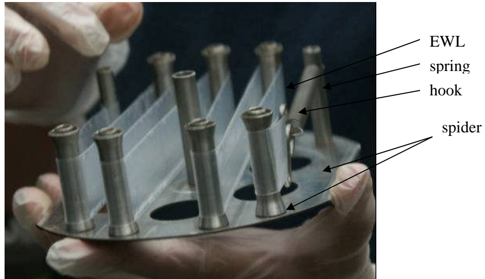
Stainless steel spider with the mounted EWL - Exposmeter Lipophilic for water
