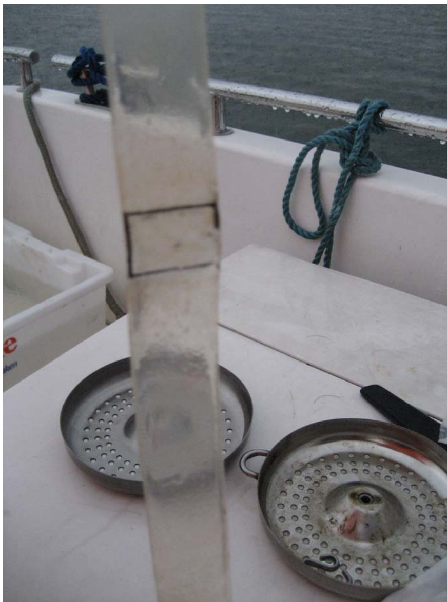
Figure 6. Example on EHD membrane retrieved from the Oslo fjord after 21 days of exposure.
