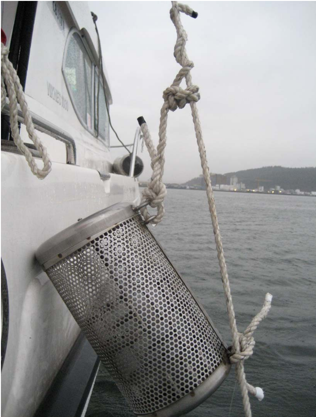
Figure 3. Commercially available stainless steel SPMD deployment apparatus: On the picture is a protective stainless steel cage for five SPMD spiders attached to ropes for being submerged into the Oslo fjord.
