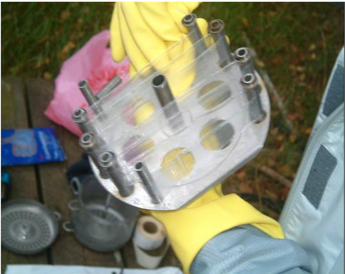
Figure 2. Standard SPMD configuration before deployment. A 92 cm membrane is applied to the stainless steel spider before placement in the protective stainless steel device.
