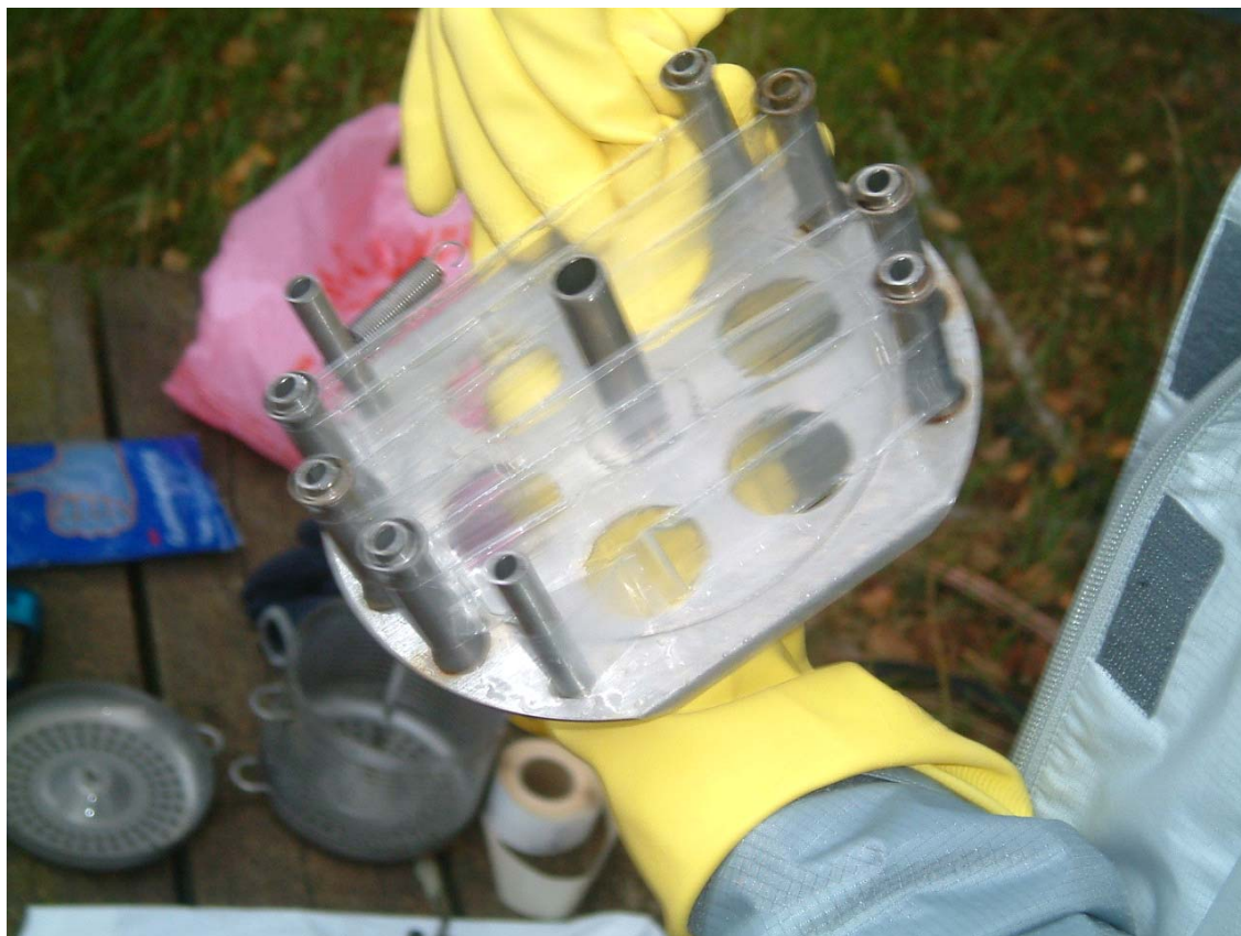
FIGURE 3. STANDARD SPMD CONFIGURATION BEFORE DEPLOYMENT. A 92 CM MEMBRANE IS APPLIED TO THE STAINLESS STEEL SPIDER BEFORE PLACEMENT IN THE PROTECTIVE STAINLESS STEEL DEVICE.
