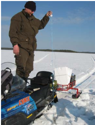
Figure 5. Sampling in deep areas. EMDs tighten to the rope at the different levels.
